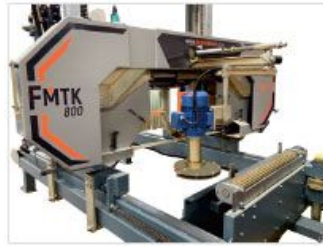
Band saw stabilizer / Cutting line cleaner Şerit testere sabitleyici / Ön kesici
